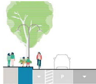
Expand the furnishing zone to include seating, shade, bike racks and micro-mobility parking, and increased street greening and wayfinding
